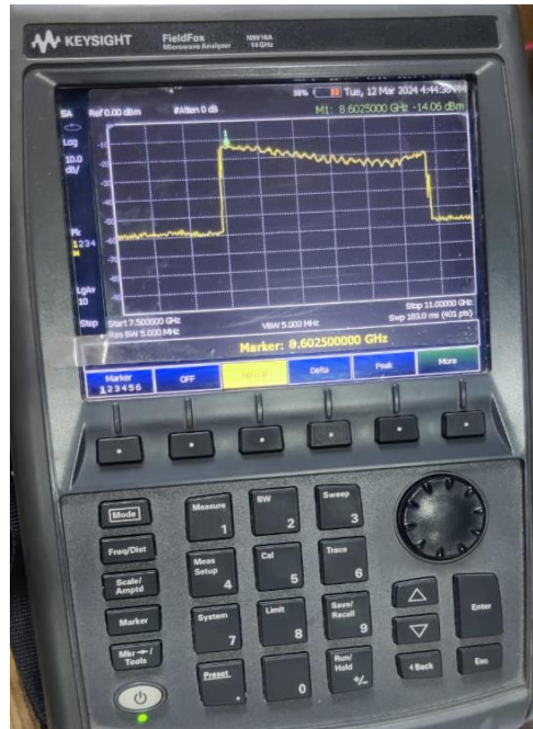
Fig 6. Bandwidth of X-Band
